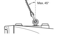
**Incorrect:** Do not suspend the eye bolts as shown in the illustrations below.
